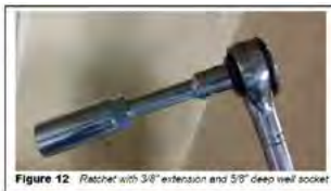
Figure 12 Ratchet with 3" extension and 5/8" deep well socket
